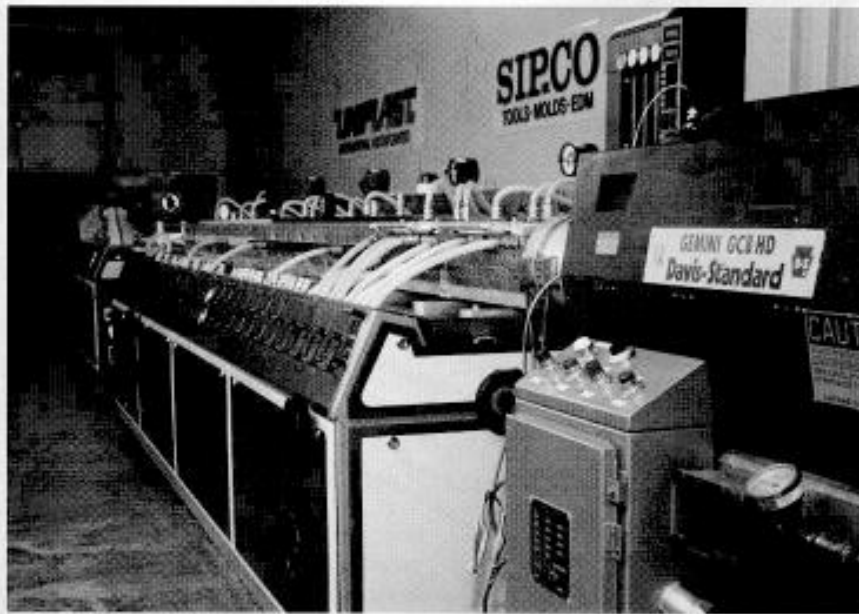
Fig. 4-20. Profile extrusion line. (Courtesy Davis-Standard)
