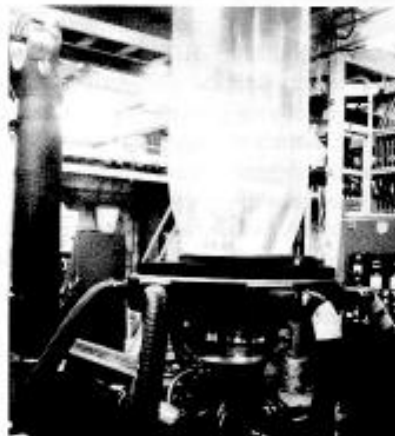
Figs. 4-11 and 4-12. Blown film process. (Courtesy Davis-Standard)
