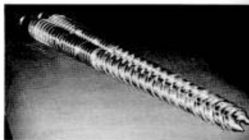
Fig. 4-7. Conical twin screws. (Courtesy Davis-Standard)
